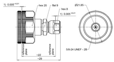
1) Pin depth (inner conductor recessed)
