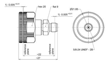
1) Pin depth (inner conductor recessed)
