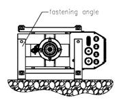
e.g. horizontal installation, cooling air flow upwards
