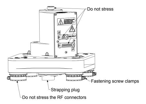
Use transportation and lifting gear approved to carry at least 10 kg only. Do not stress the connectors and the manual override.
