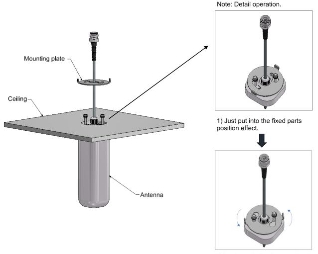
2) As shown in the figure, rotate the fixing parts to clamp the antenna screws.
