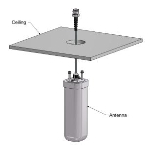
Step 3: Route the antenna cable through the mounting plate and attach it to the ceiling surface.
